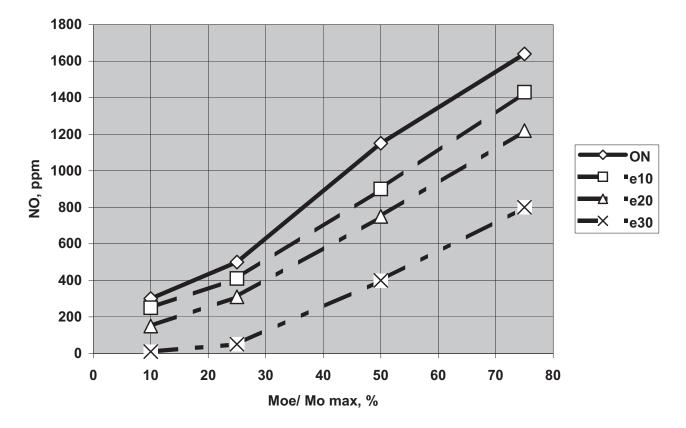
Fig. 6. Concentration of  $NO_x$  in exhaust gases in the function of the engine load for different water proportions in the emulsion fuel: ON – diesel oil, e10 - 30 emulsion fuel of water content 10 - 30%
