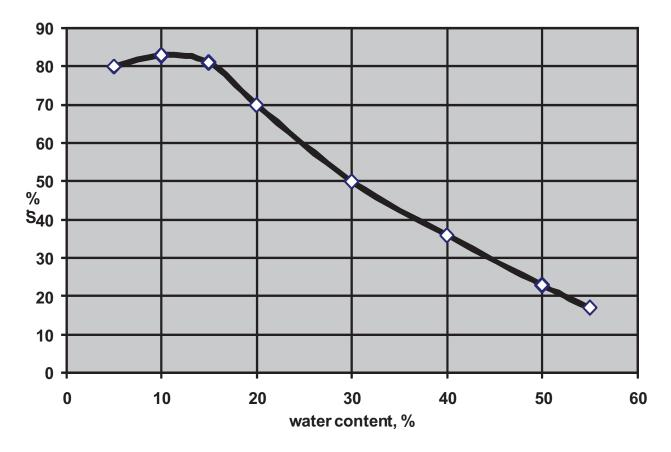
Fig. 1. The effect of water proportion in fuel on the change of the engine smoking [1]
