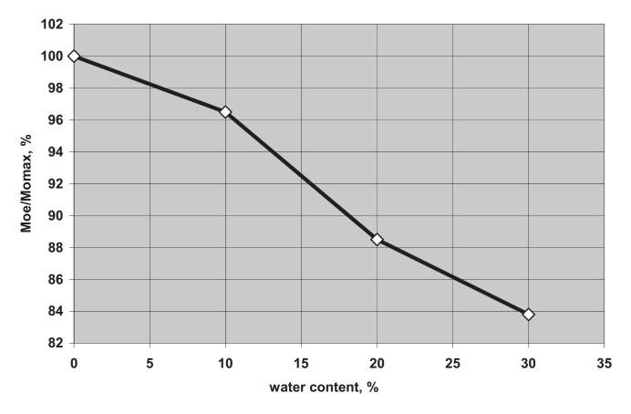
Fig. 4. The effect of water proportion in the emulsion fuel on the relative value of the engine torque
