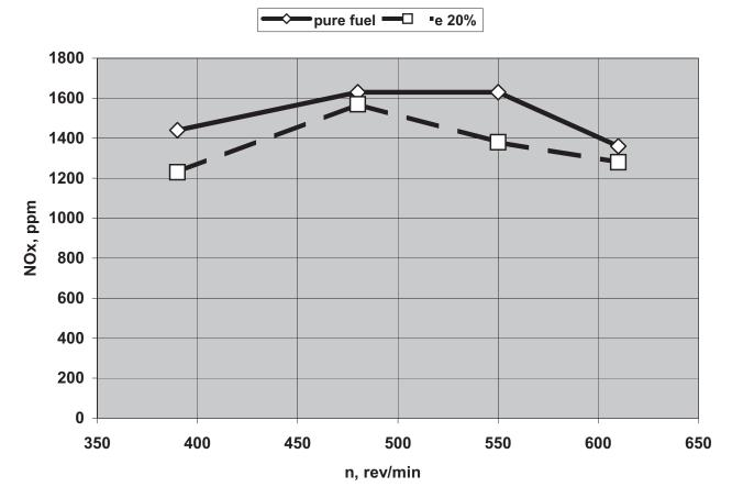
*Fig. 3. Concentration of NOx in the function of rotational speed for standard fuel and emulsion fuel of 20% water content [8]*
