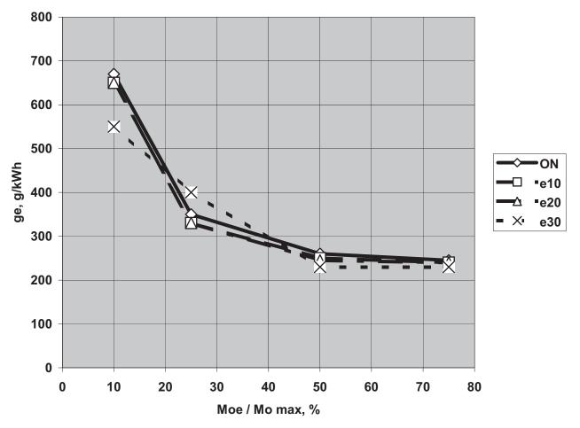
Fig. 7. Unit fuel consumption in the function of the engine load for different water proportions in the emulsion fuel: ON – diesel oil, e10 - 30 emulsion fuel of water content 10 - 30%
