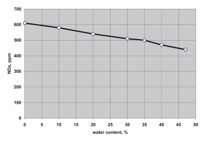
*Fig. 2. Concentration of NOx in exhaust gases in the function of water proportion of water injected to the suction manifold [6]*
